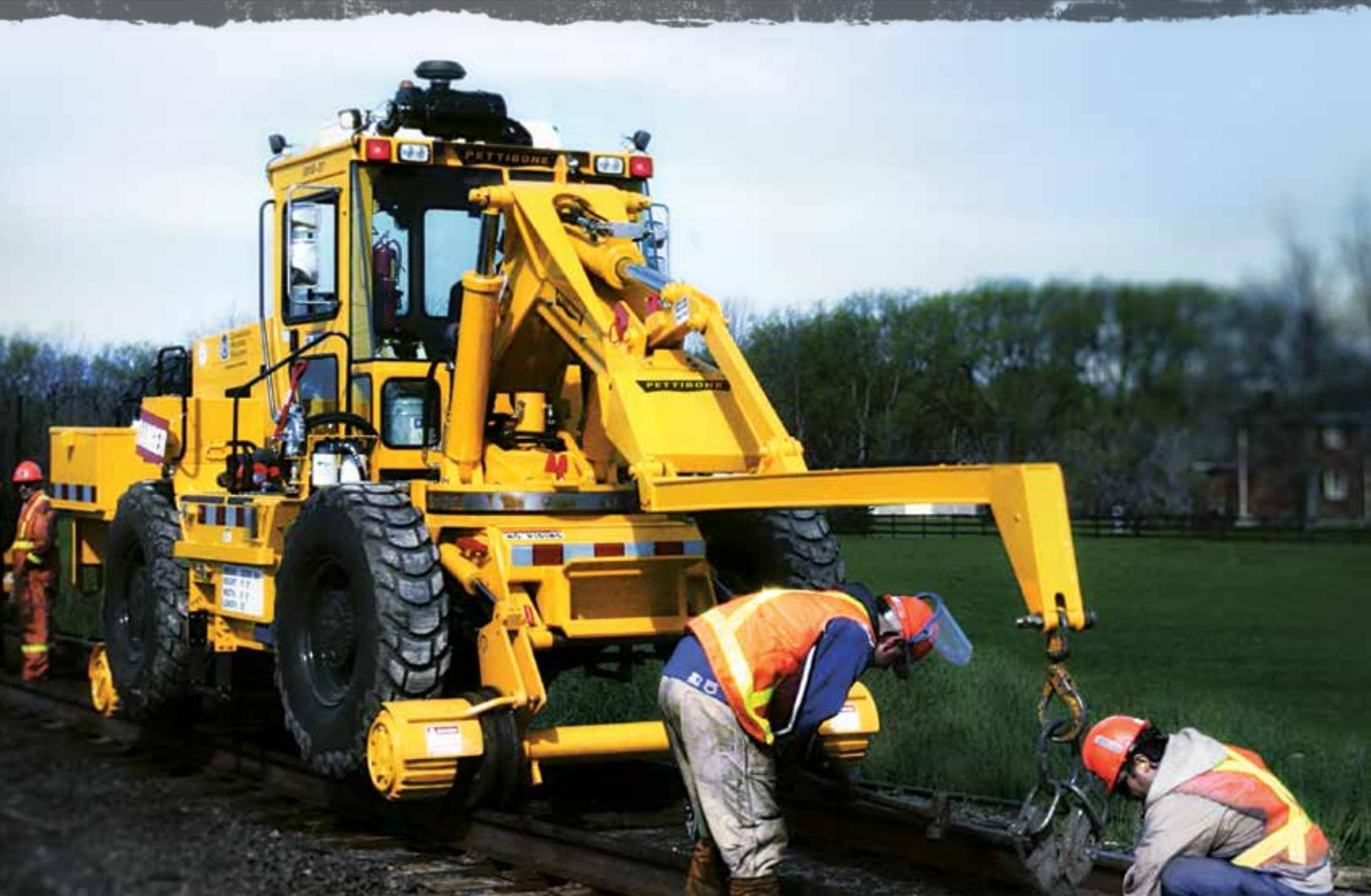
Designed to tackle a variety of rail applications, the Pettibone® Speed Swing™ 445E is a versatile machine that provides the power to lay rails, set ties or clear the path ahead. The unit features a turbo diesel engine and 180-degree boom rotation for enhanced productivity. Offering precise hydraulics, numerous attachments and the ability to work both on and off the rails, the Speed Swing 445E is equipped for any rail task.
